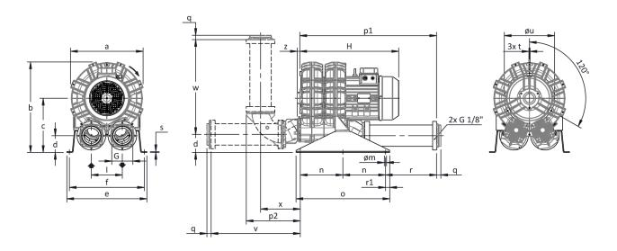
Configuration with a vertical silencer is only available with the CK accessory kit; for all assembly options refer to FPZ. Dimensions in mm NOT Binding
